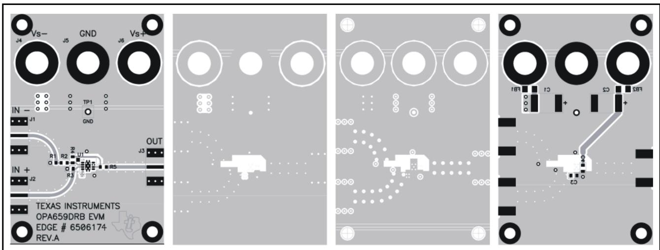
Figure 27. OPA653EVM PCB Layers 1 through 4
