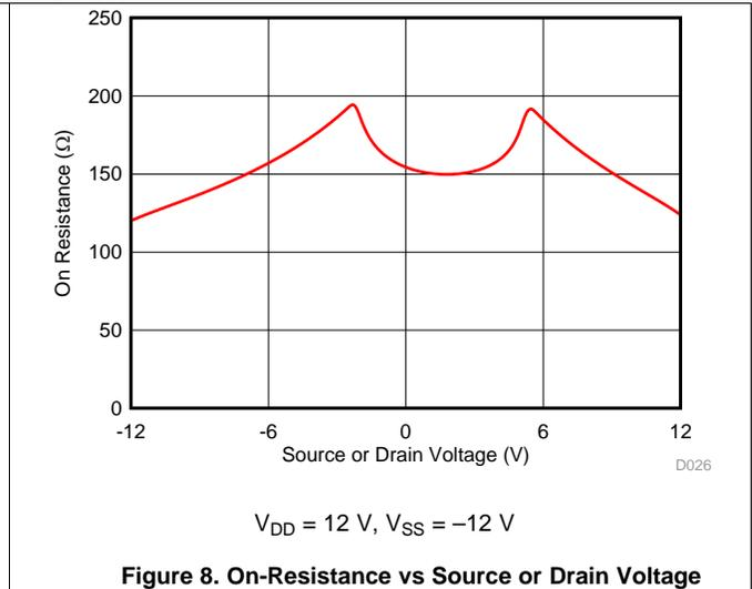
Figure 8. On-Resistance vs Source or Drain Voltage
