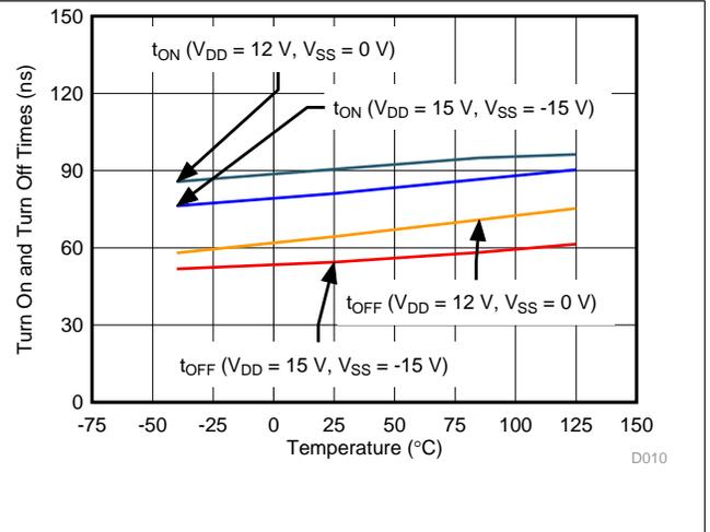
Figure 14. Turn-On and Turn-Off Times vs Temperature
