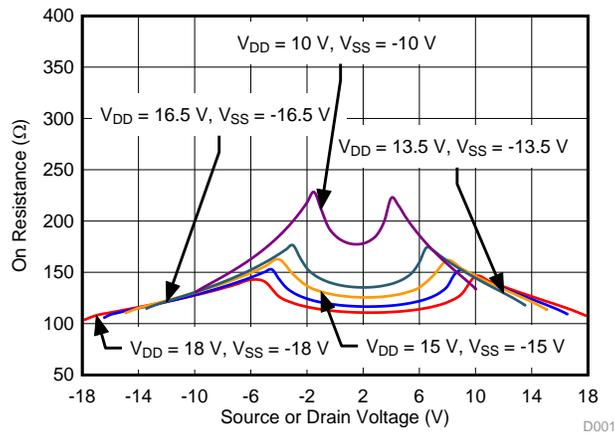
**Figure 44. On-Resistance Variation With Supply and Input Voltage**
