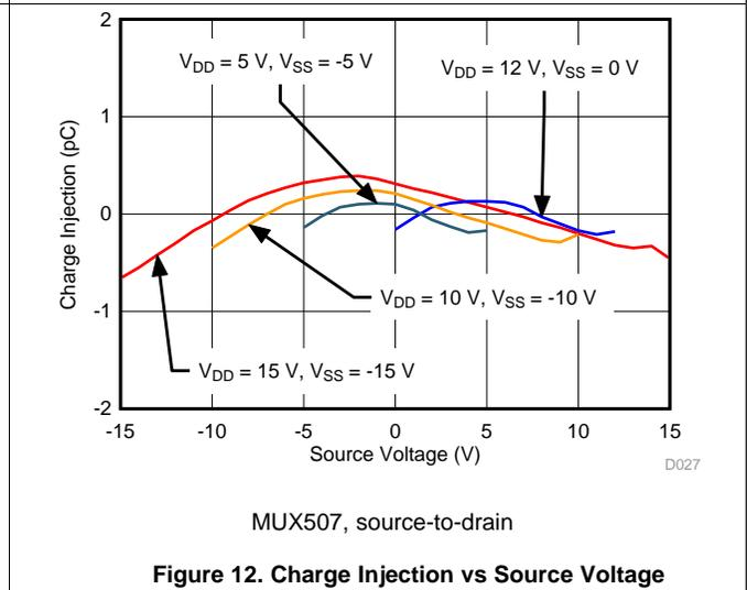
Figure 12. Charge Injection vs Source Voltage
