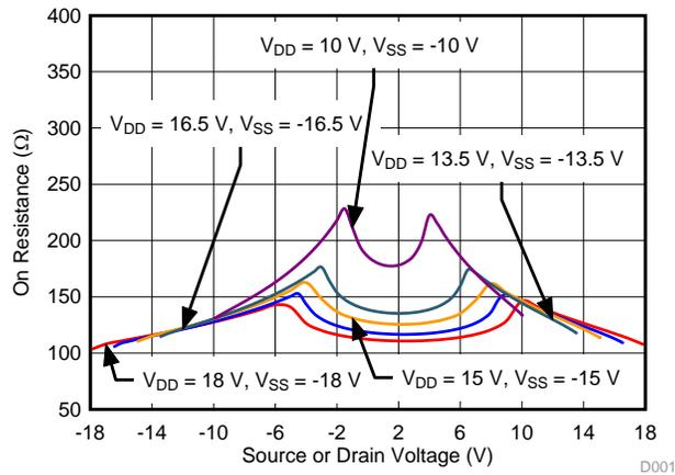
Figure 41. On-resistance vs Source or Drain Voltage
