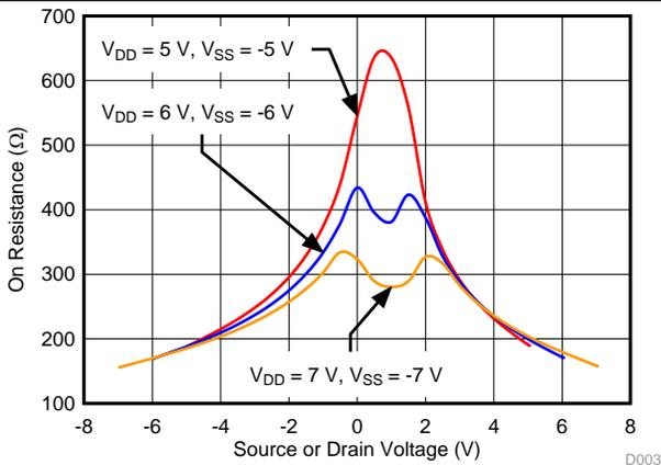
Figure 3. On-Resistance vs Source or Drain Voltage
