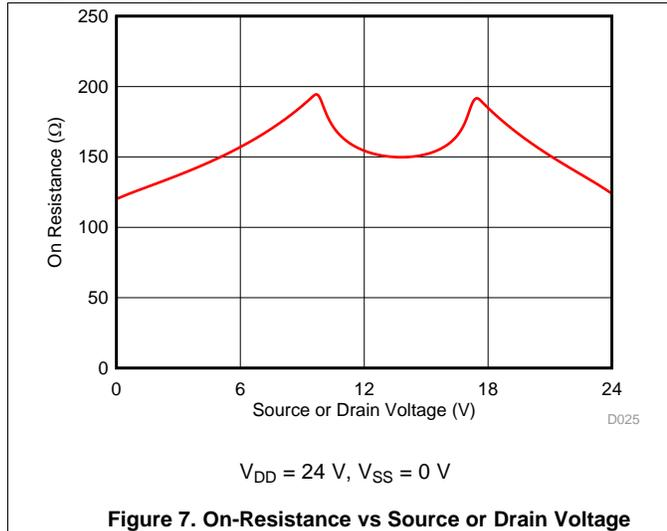
Figure 7. On-Resistance vs Source or Drain Voltage
