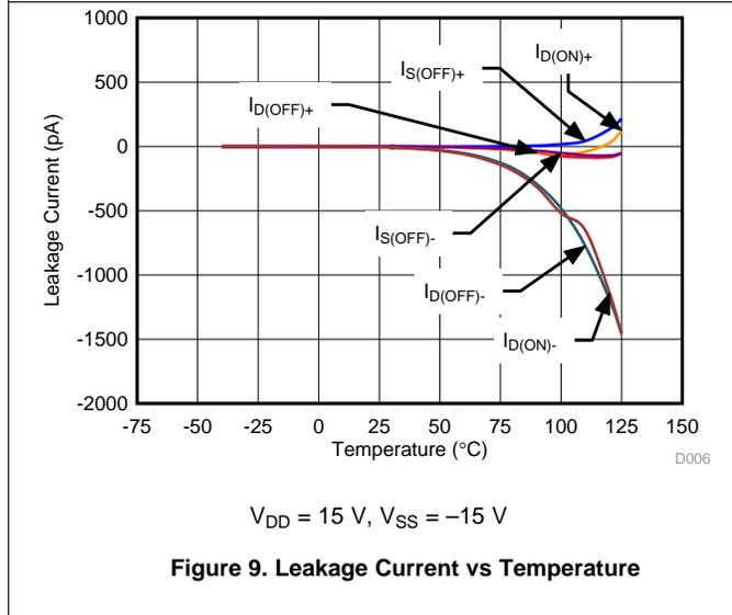
Figure 9. Leakage Current vs Temperature
