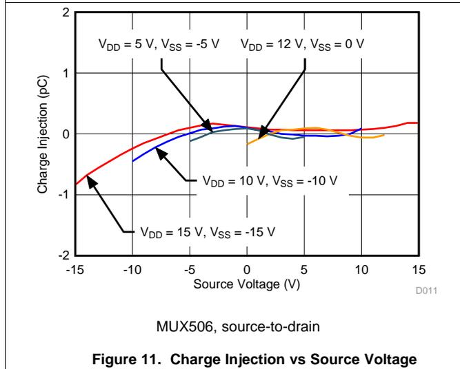
Figure 11. Charge Injection vs Source Voltage
