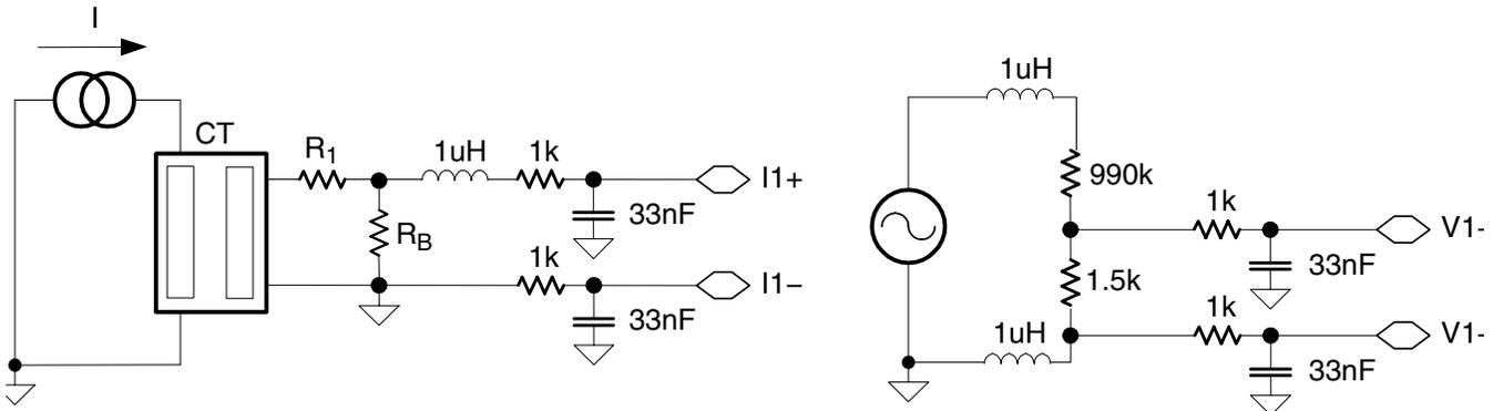
Figure 14. Energy Measurement Test Circuitry (SD16GAINx = 1)
