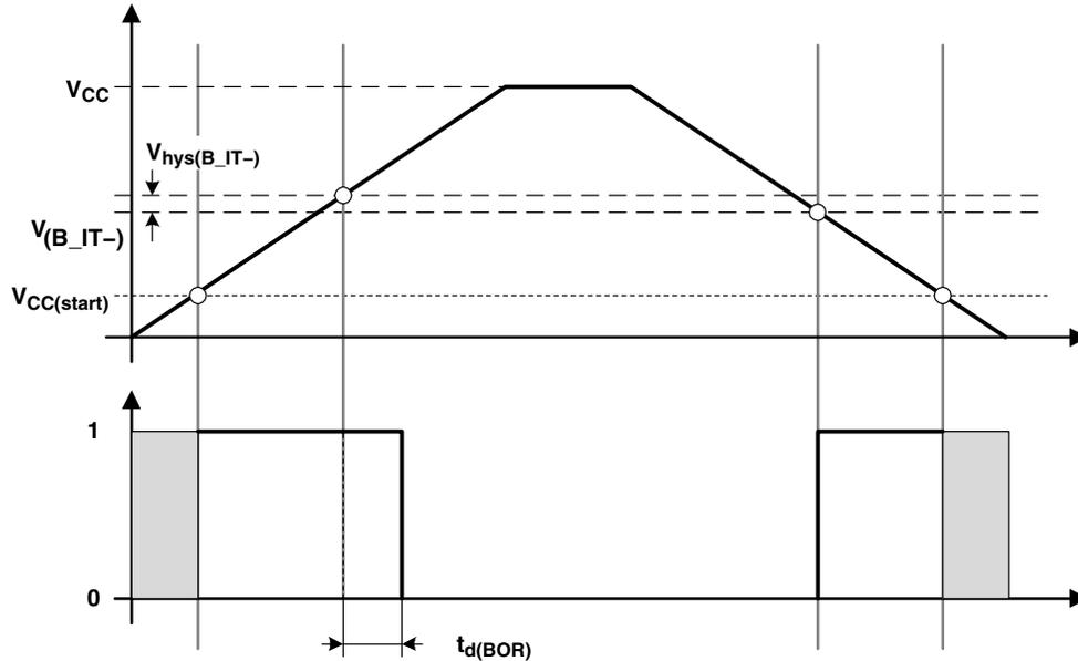
Figure 6. POR/Brownout Reset (BOR) vs Supply Voltage
