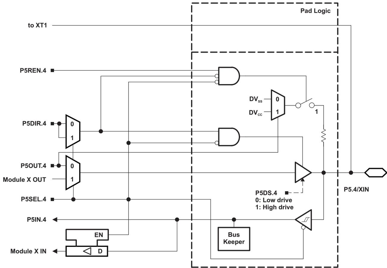
Port P5, P5.7, Input/Output With Schmitt Trigger
