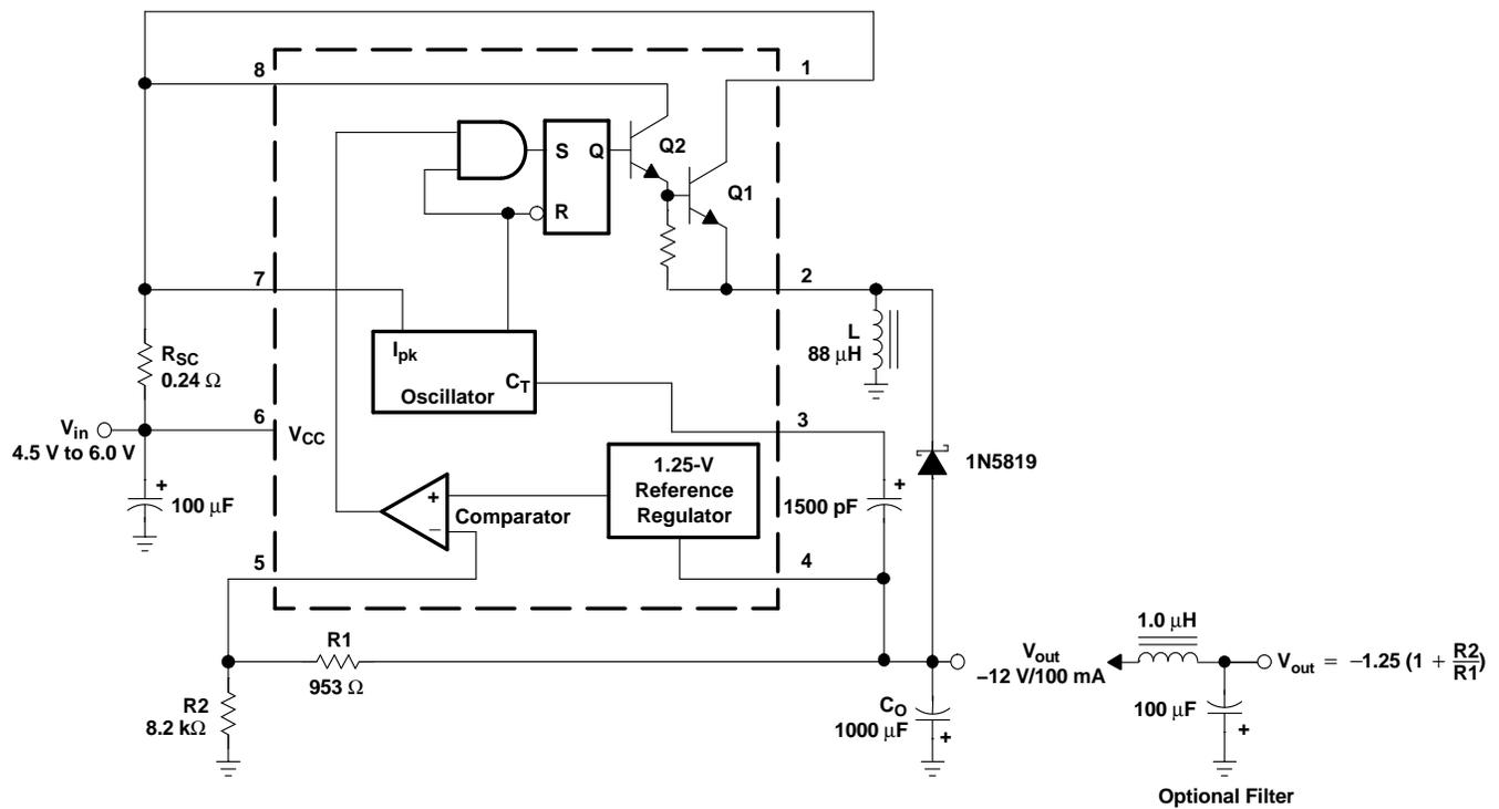
Figure 10. Voltage-Inverting Converter
