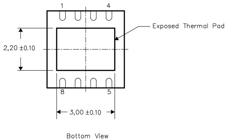
NOTE: All linear dimensions are in millimeters
