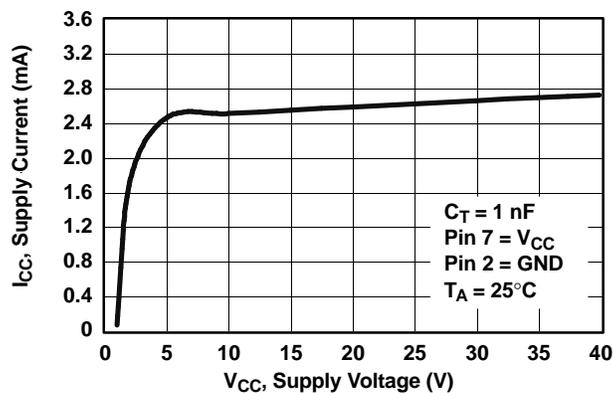
Figure 5. Standby Supply Current vs Supply Voltage
