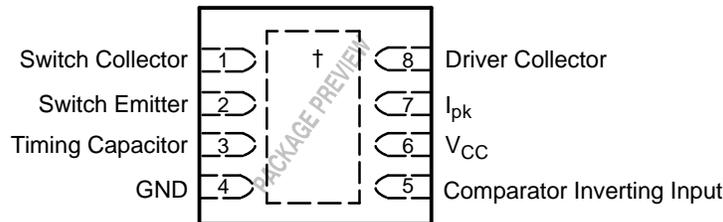
† Exposed thermal pad is connected internally to GND via die attach.
