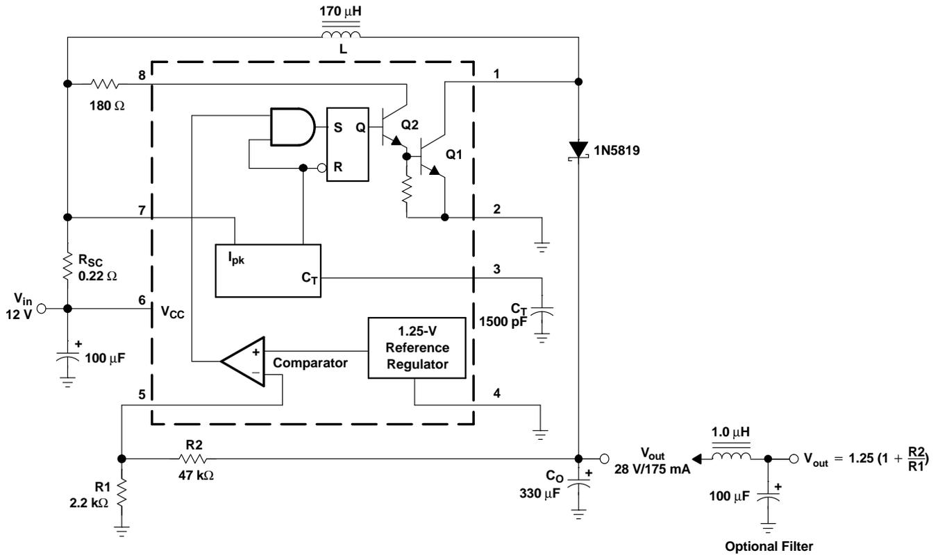
Figure 6. Step-Up Converter
