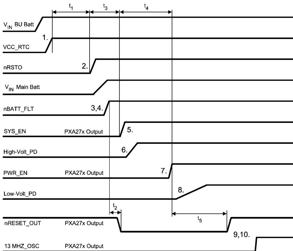
\* Note that BOTH nRSTO and nBATT\_FLT need to be de-asserted before SYS\_EN is enabled. The sequence of the two signals is independent of each other and can occur in either order.
