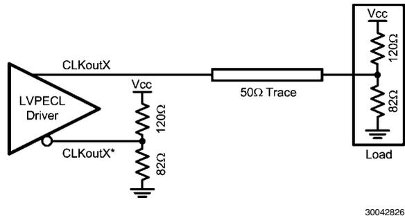
**FIGURE 9. Single-Ended LVPECL Operation, DC Coupling, Thevenin Equivalent**
