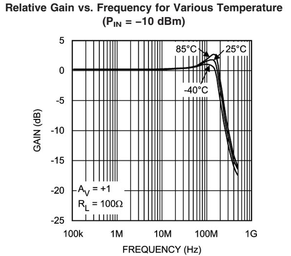
**Typical Performance Characteristics** At  $T_J = 25^\circ\text{C}$ ,  $V^+ = 16\text{ V}$ ,  $V^- = 0\text{ V}$ ,  $R_F = 330\Omega$  for  $A_V = +2$ ,  $R_F = 1\text{ k}\Omega$  for  $A_V = -1$ .  $R_L$  tied to  $V^+/2$ . Unless otherwise specified. (Continued)
