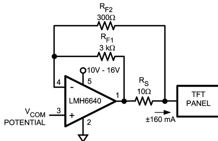
Typical Application as a TFT Panel V<sub>COM</sub> Driver
