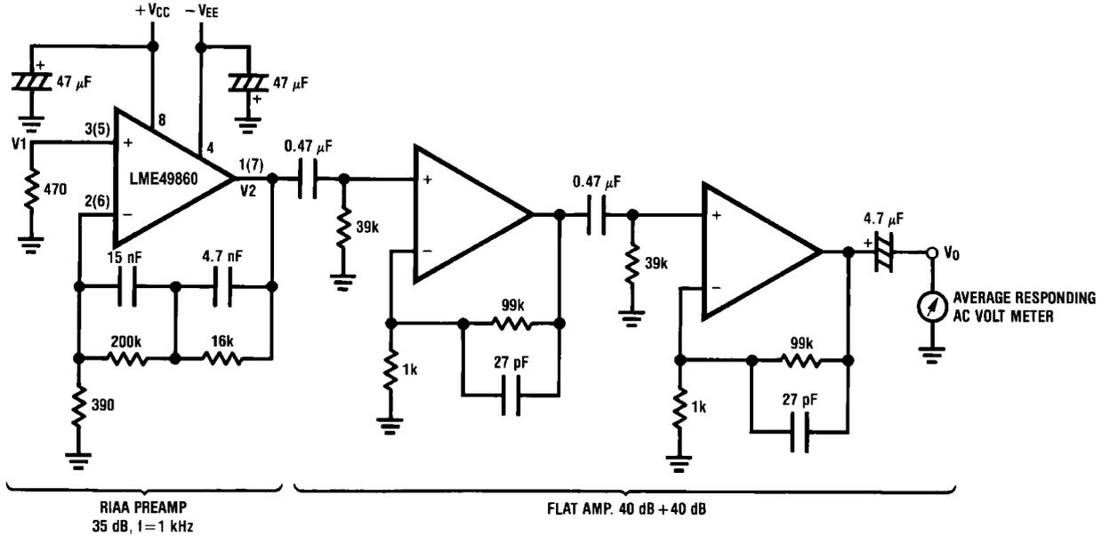
Complete shielding is required to prevent induced pick up from external sources. Always check with oscilloscope for power line noise.
