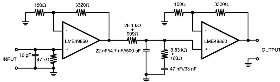
Note: 1% metal film resistors, 5% polypropylene capacitors
