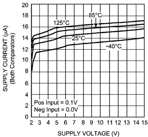
Supply Current vs. Supply Voltage (Output Low)
