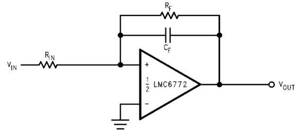
**FIGURE 3. Canceling the Effect of Input Capacitance**
