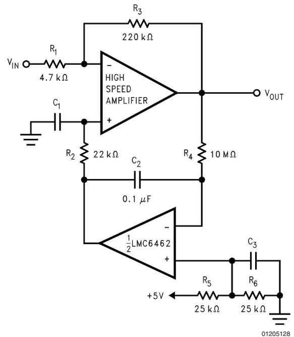
FIGURE 22. High Gain Amplifier with Low Frequency Null
