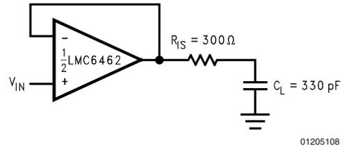
**FIGURE 4. Resistive Isolation of a 300 pF Capacitive Load**
