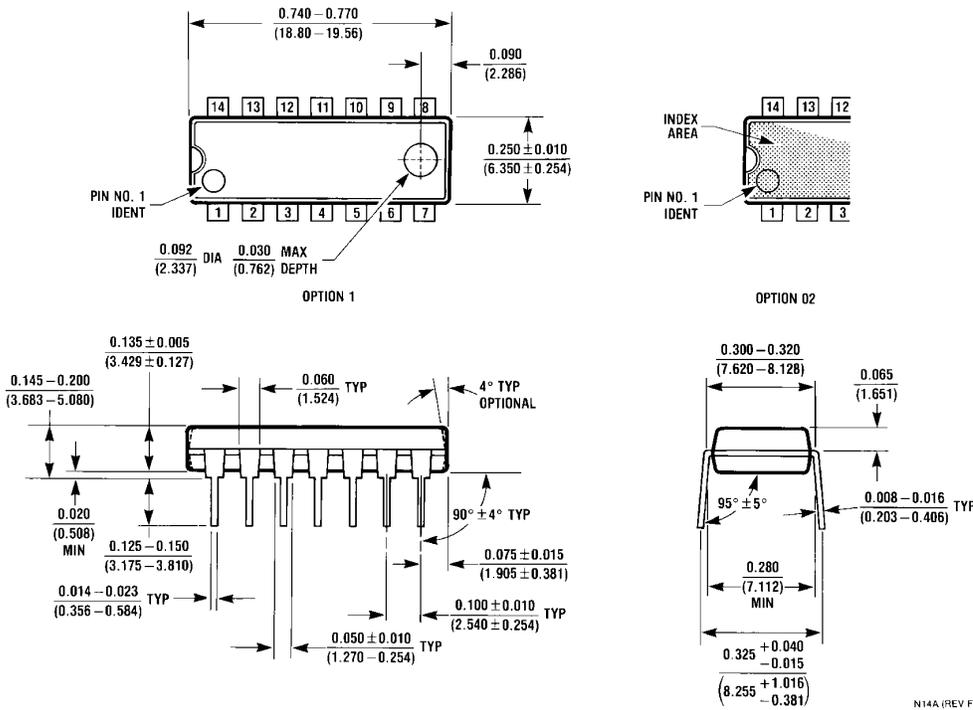
**14-Pin Molded Dual-In-Line Package**
