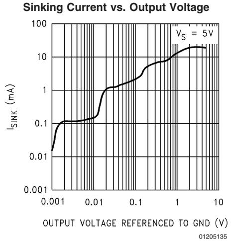
**Typical Performance Characteristics**  $V_S = +5V$ , Single Supply,  $T_A = 25^\circ C$  unless otherwise specified (Continued)
