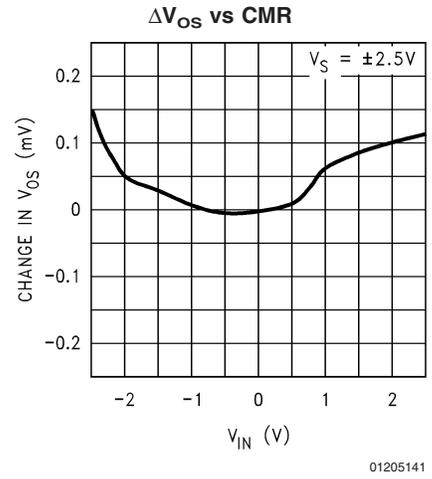
**Typical Performance Characteristics**  $V_S = +5V$ , Single Supply,  $T_A = 25^\circ C$  unless otherwise specified (Continued)
