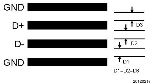
FIGURE 4. Ideal Diode Trace Layout
