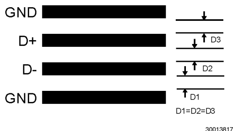
FIGURE 9. Ideal Diode Trace Layout
