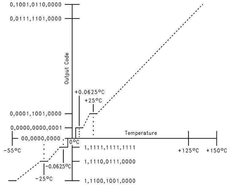
Figure 5. Temperature-to-Digital Transfer Function (Non-linear scale for clarity)
