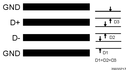
FIGURE 15. Ideal Diode Trace Layout
