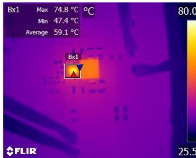
Figure 13. Thermal Image Capture of IC at VIN = 13.5 V, VOUT = 5 V, Load = 6 A
