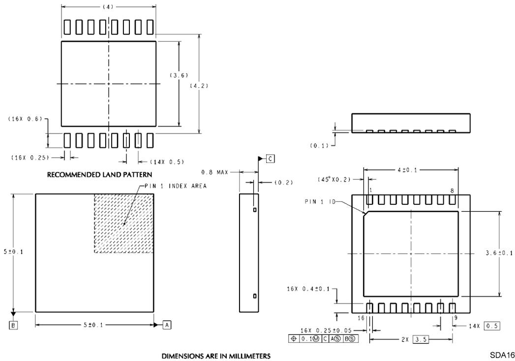
Note: It is recommended that the exposed pad be connected to Pin 11 (AGND)
