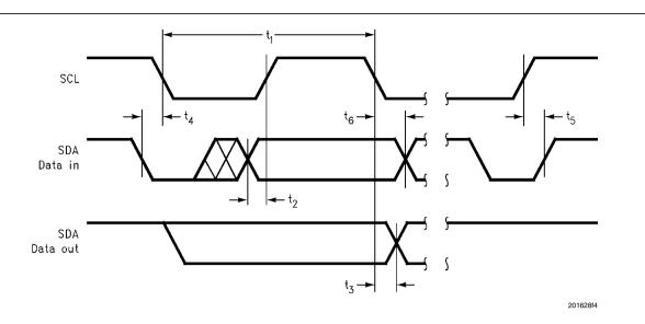
FIGURE 4. I<sup>2</sup>C Timing Diagram
