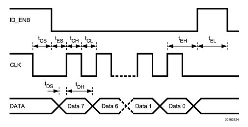
FIGURE 5. SPI Timing Diagram
