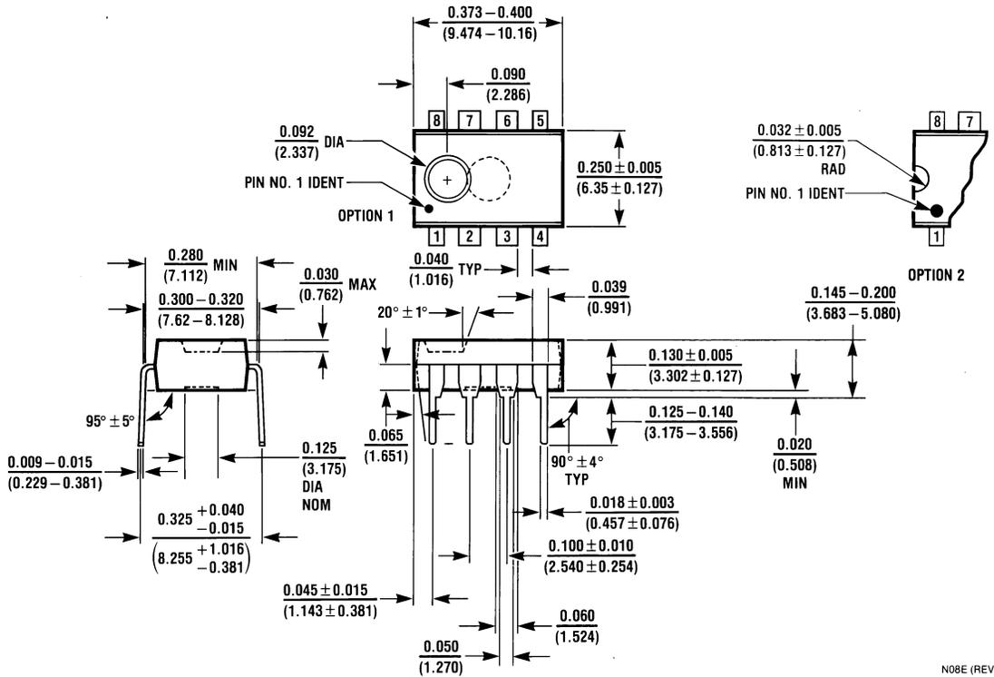
**8-Lead (0.300" Wide) Molded Dual-In-Line Package**
