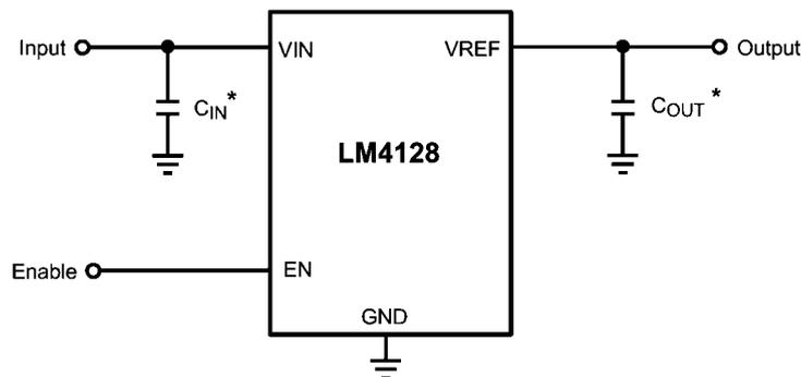
\*Note: The capacitor  $C_{IN}$  is required and the capacitor  $C_{OUT}$  is optional.
