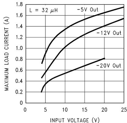
**Figure 45. Maximum Load Current for Inverting Regulator Circuit**
