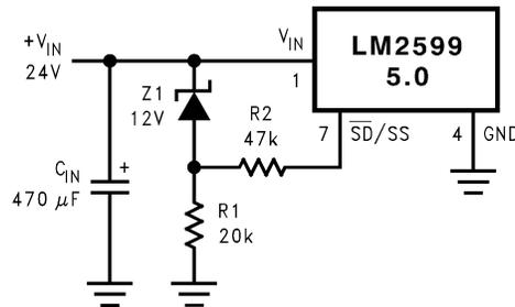
**Figure 46. Undervoltage Lockout for a Buck Regulator**
