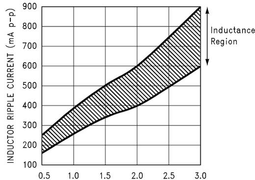
**Figure 37. Peak-to-Peak Inductor Ripple Current vs Load Current**
