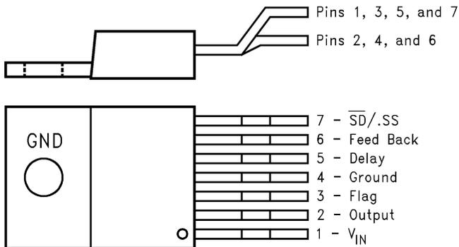
**Figure 1. Bent and Staggered Leads, Through Hole Package**
