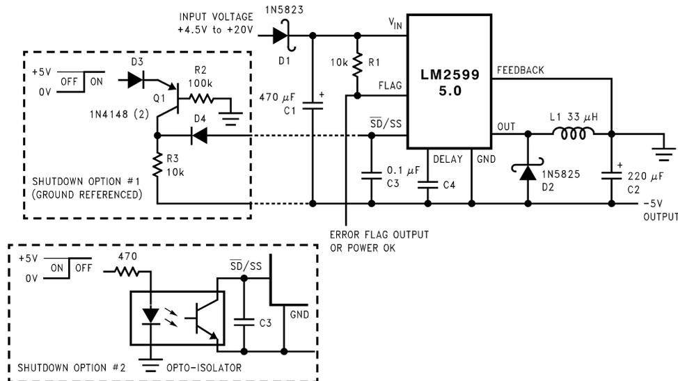
**Figure 43. Inverting -5V Regulator With Shutdown and Soft-start**
