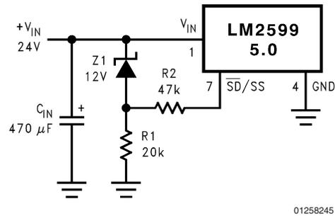
**FIGURE 29. Undervoltage Lockout for a Buck Regulator**
