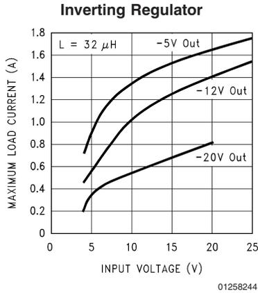
**FIGURE 28. Maximum Load Current for Inverting Regulator Circuit**
