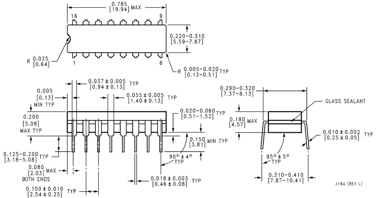
**16-Lead Ceramic Dual-in-Line Package (J)**
