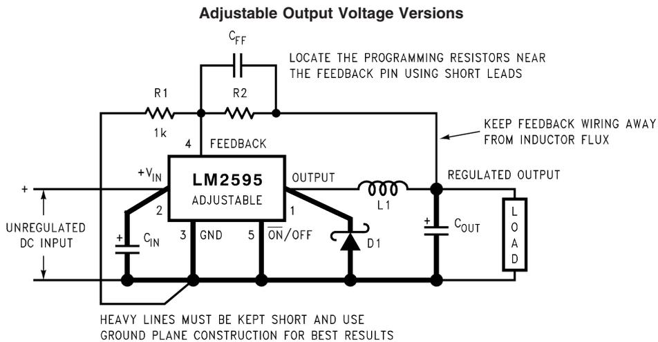
$$V_{OUT} = V_{REF} \left( 1 + \frac{R_2}{R_1} \right) \quad \text{where } V_{REF} = 1.23V$$
