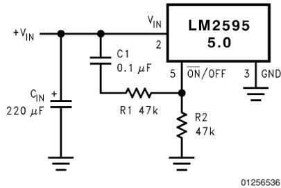
FIGURE 21. Delayed Startup
