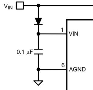
**Figure 28. Input Blocking Diode for VCCX > VIN**
