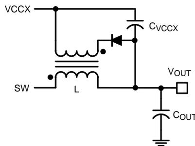
**Figure 27. VCCX Bias Supply with Additional Inductor Winding**
