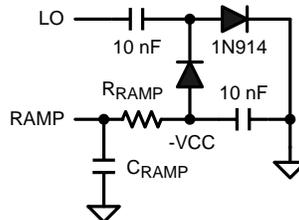
**Figure 40.  $R_{\text{RAMP}}$  to -VCC for  $V_{\text{OUT}} < 7.5\text{V}$**
