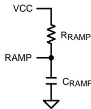
**Figure 39.  $R_{\text{RAMP}}$  to VCC for  $V_{\text{OUT}} > 7.5\text{V}$**
