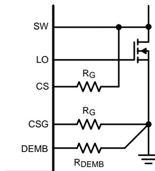
Figure 32.  $R_{DS(ON)}$  Current Sensing without Diode Emulation
