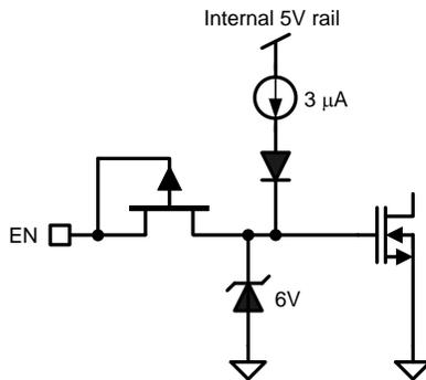
Figure 29. Enable Circuit
