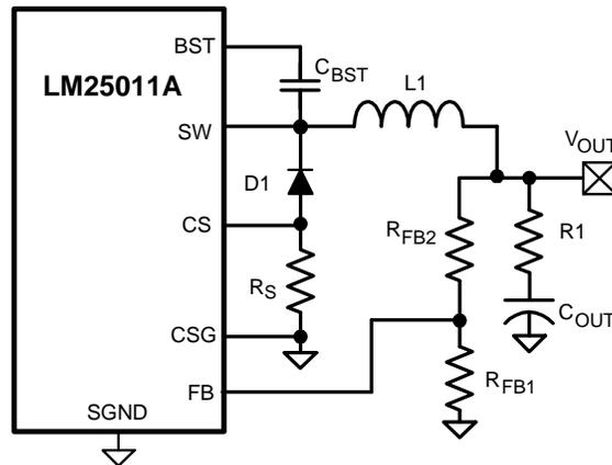
**Figure 22. Option A – Lowest Cost Ripple Configuration**
