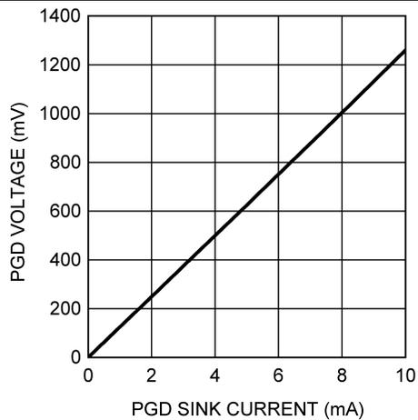
**Figure 7. PGD Low Voltage vs Sink Current**
