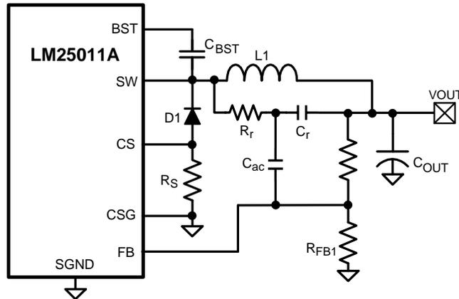
**Figure 24. Option C: Minimum Output Ripple Configuration**
