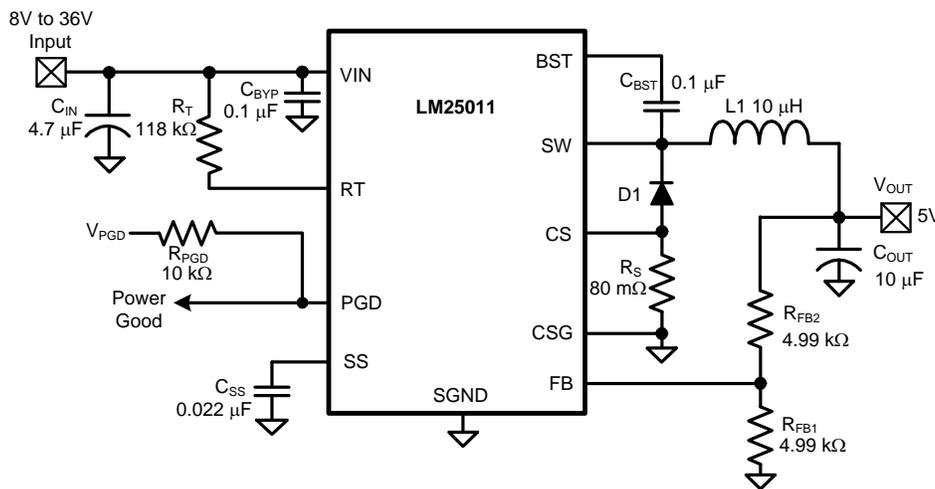
Figure 19. Example Circuit
