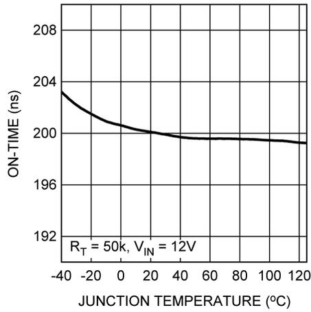
Figure 13. On-Time vs Temperature
