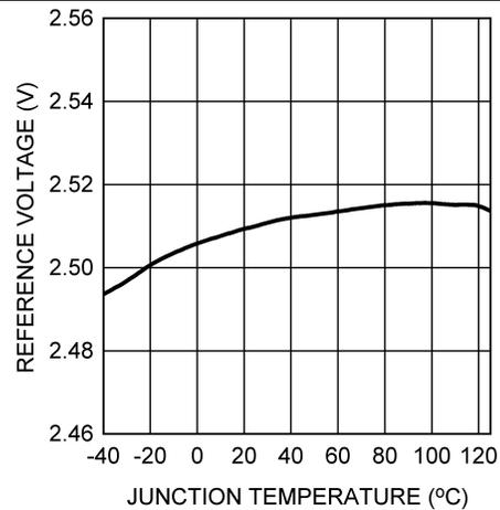
**Figure 8. Reference Voltage vs Temperature**
