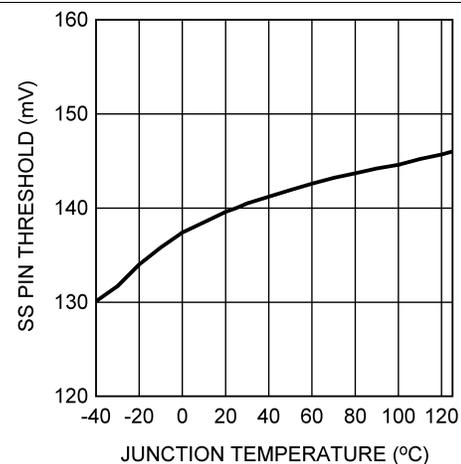
**Figure 12. SS Pin Shutdown Threshold vs Temperature**
