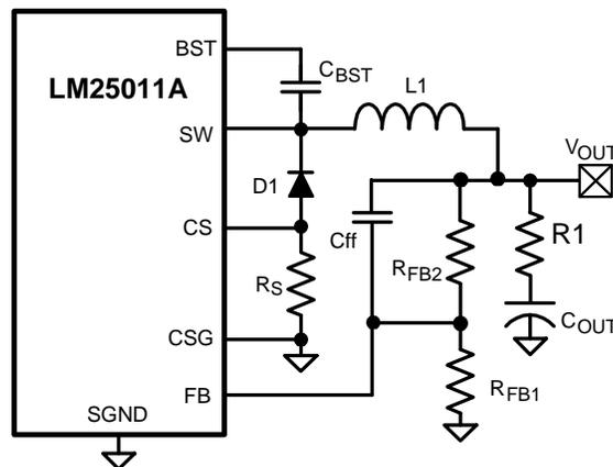
**Figure 23. Option B – Intermediate Ripple Configuration**
