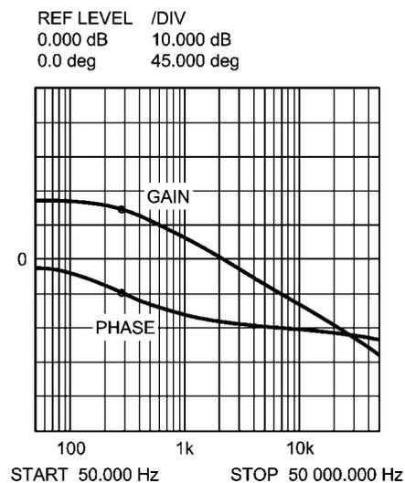
**FIGURE 9. Gain and Phase of Modulator**
