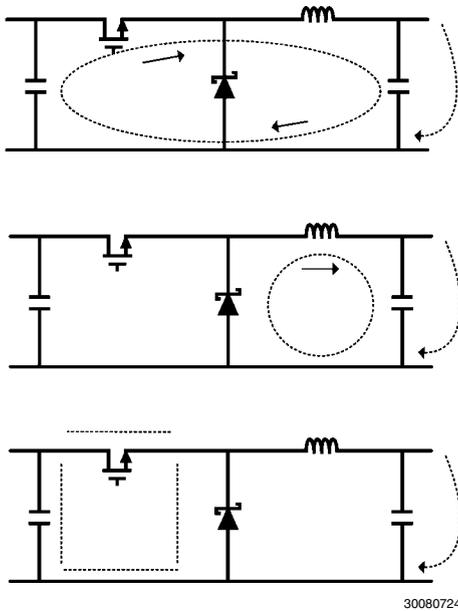
FIGURE 11. Current Flow in a Buck Application
