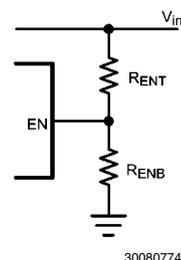
FIGURE 2. External UVLO Connections
