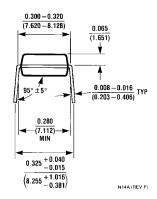
Molded Dual-In-Line Package (N) Order Number LM1877N-9 NS Package Number N14A
