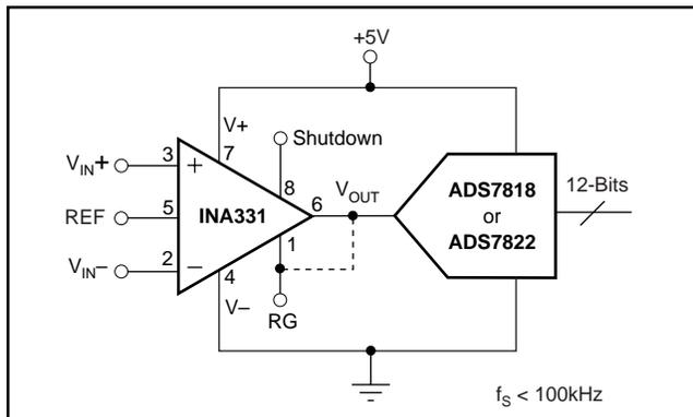
FIGURE 4. INA331 Directly Drives Capacitive-Input, High-Speed A/D Converter.
