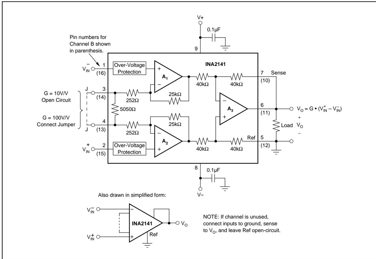
FIGURE 1. Basic Connections.
