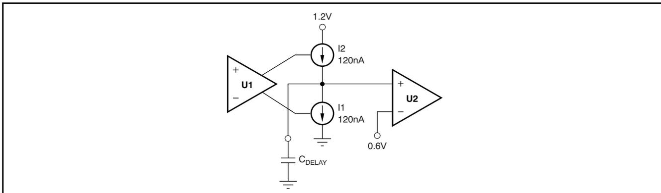
Figure 34. Simplified Model of the Comparator 2 Delay Circuit
