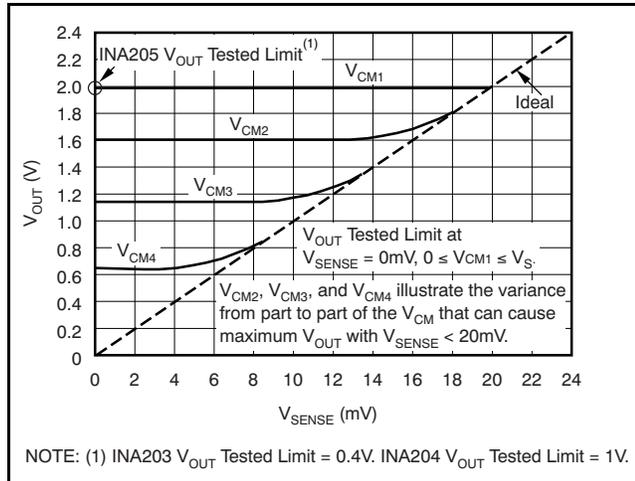
**Figure 32. Example for Low  $V_{SENSE}$  Case 2 (INA205, Gain = 100)**
