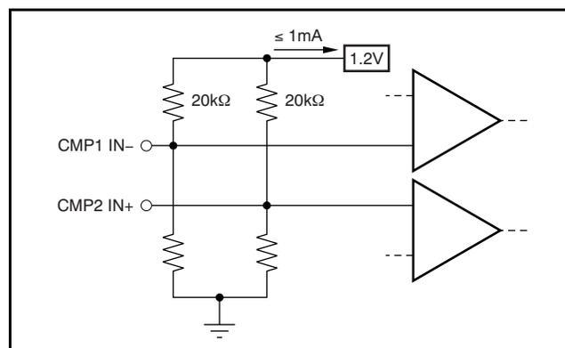
Figure 36. Limit Current Into Reference ≤ 1mA
