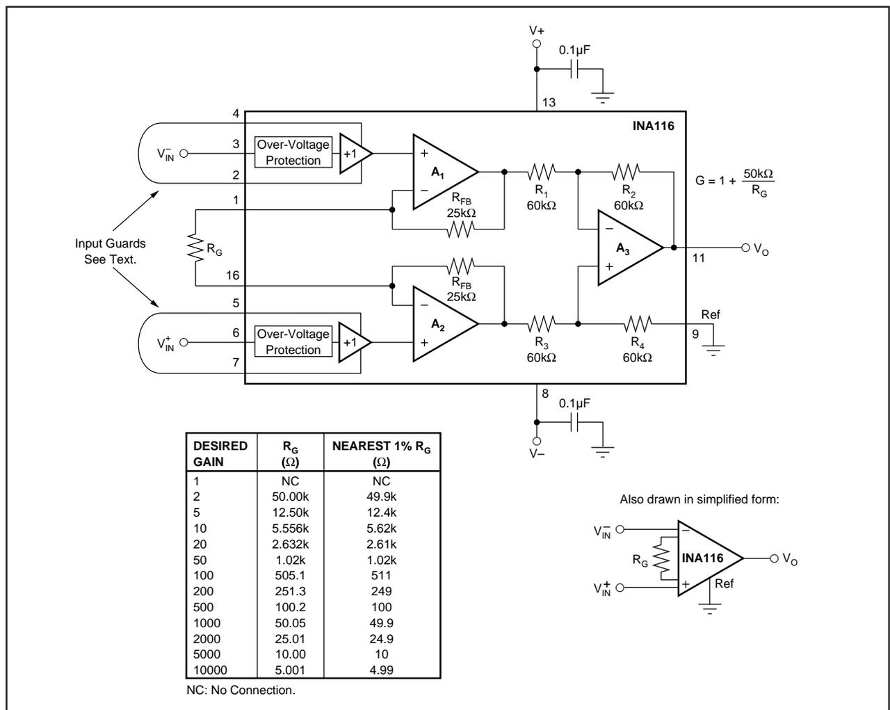
FIGURE 1. Basic Connections.
