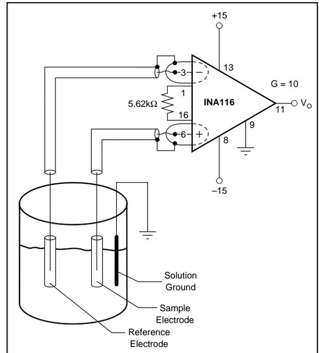
FIGURE 7. pH or Ion Measurement System.
