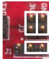
**Figure 2. USB Power Jumper Configuration**
