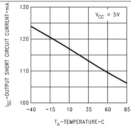
**Figure 20. Output Short Circuit Current vs Temperature**
