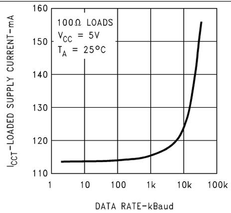
**Figure 30. Loaded Supply Current vs Data Rate**
