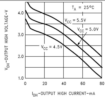
Figure 12. Output High Voltage vs Output High Current
