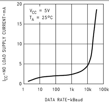
**Figure 29. No Load Supply Current vs Data Rate**
