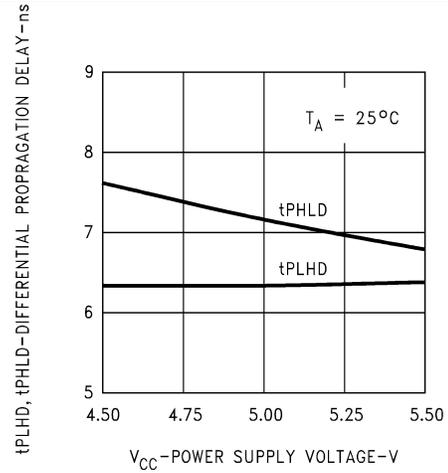
Figure 2. Differential Propagation Delay vs Power Supply Voltage
