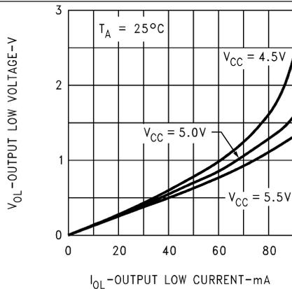
Figure 17. Output Low Voltage vs Output Low Current
