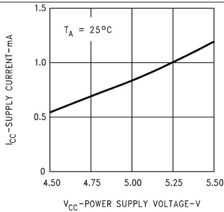
**Figure 19. Supply Current vs Power Supply Voltage**
