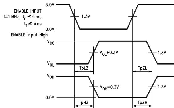
**Figure 27. Enable and Disable Times for “LS-Type” Load**
