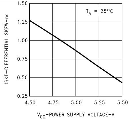
Figure 4. Differential Skew vs Power Supply Voltage
