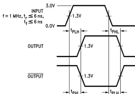
Figure 23. Propagation Delays
