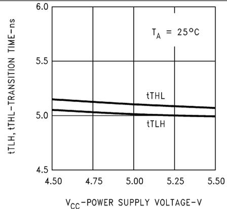
Figure 6. Differential Transition Time vs Power Supply Voltage
