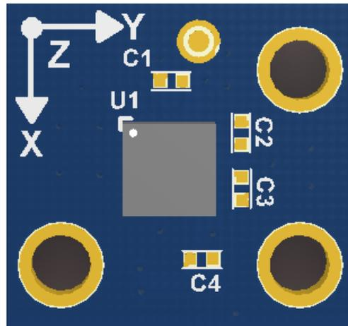
Figure 7. Acceleration Axis
