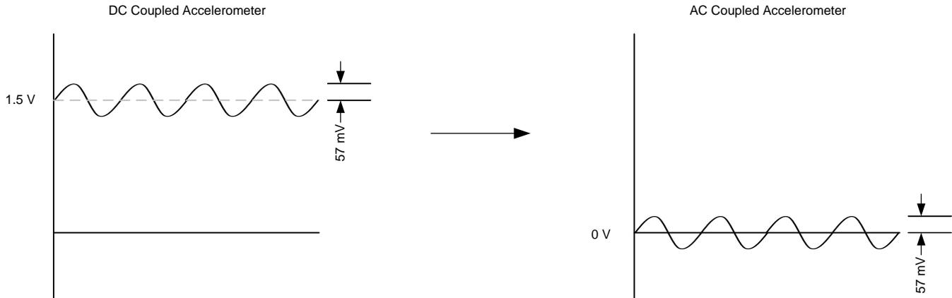
**Figure 5. AC-Coupled Accelerometer**
