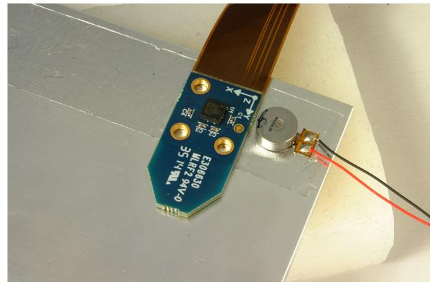
**Figure 3. Attach Accelerometer to Vibrating Object**
