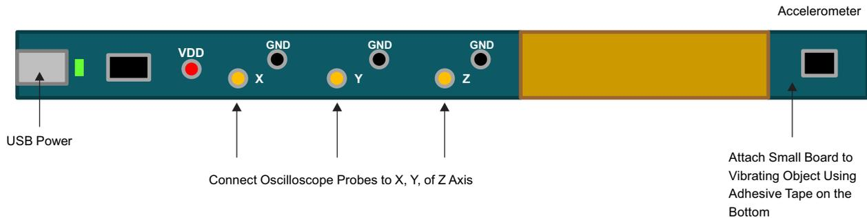
**Figure 1. Board Connections**
