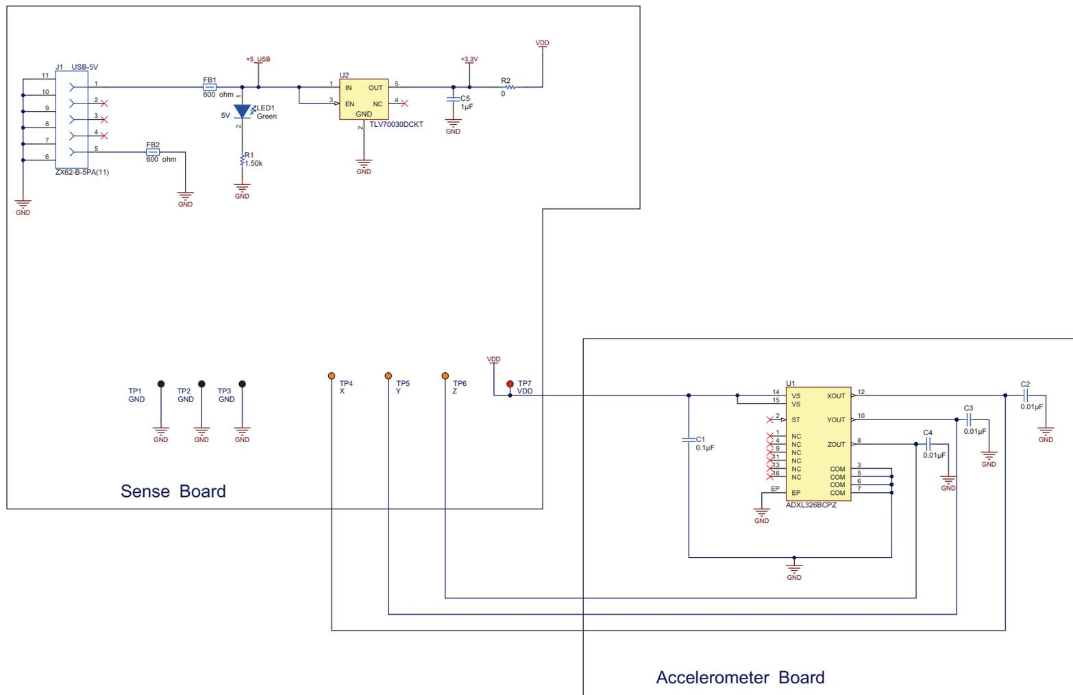
Figure 18. DRV-ACC16-EVM Schematic
