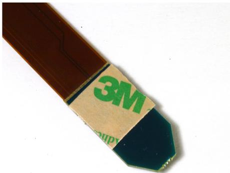
**Figure 2. 3M Tape on Backside of DRV-ACC16-EVM**
