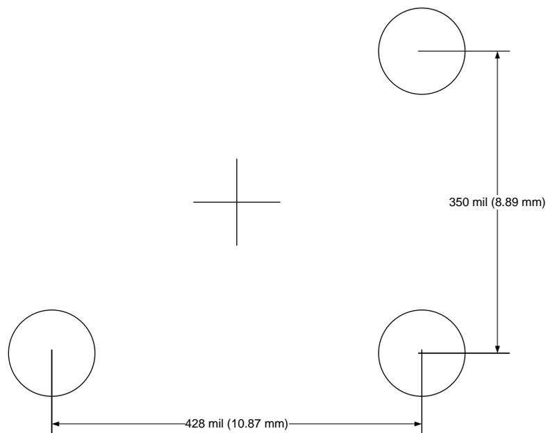
Figure 17. Screw-Hole Footprint
