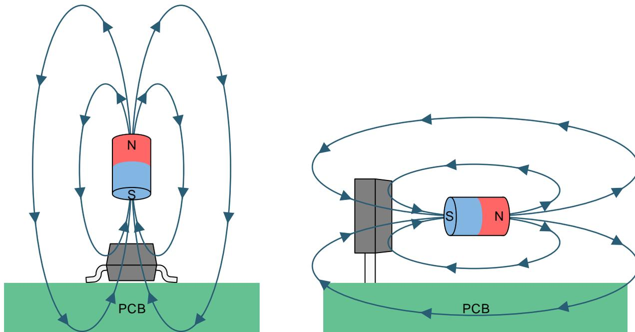
Figure 9. The Flux Direction for Positive B
