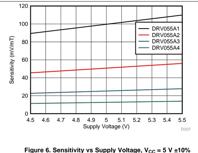
Figure 6. Sensitivity vs Supply Voltage,  $V_{CC} = 5\text{ V} \pm 10\%$
