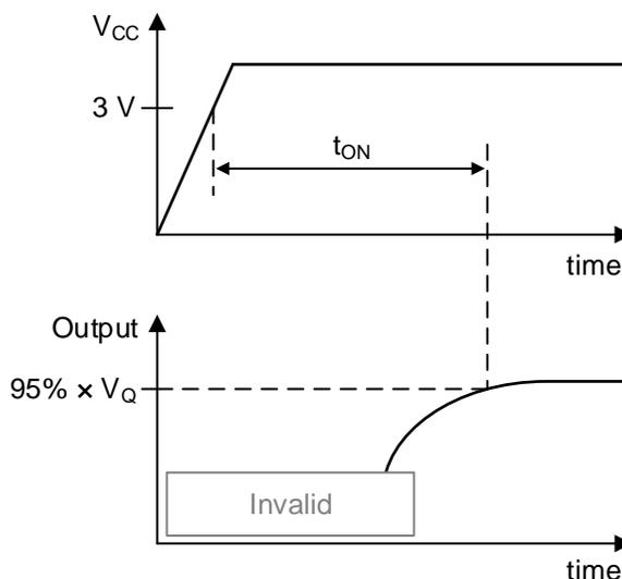
**Figure 11.  $t_{ON}$  Definition**
