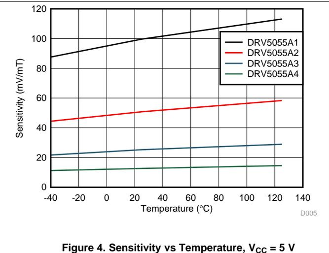
Figure 4. Sensitivity vs Temperature,  $V_{CC} = 5\text{ V}$
