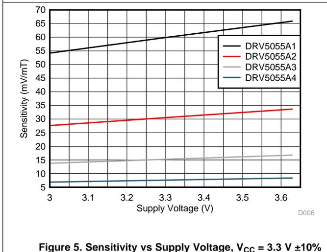
Figure 5. Sensitivity vs Supply Voltage,  $V_{CC} = 3.3\text{ V} \pm 10\%$
