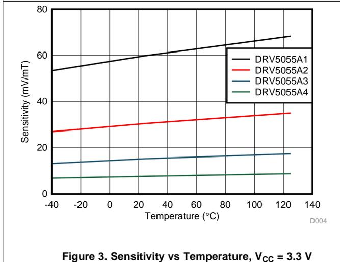
Figure 3. Sensitivity vs Temperature,  $V_{CC} = 3.3\text{ V}$
