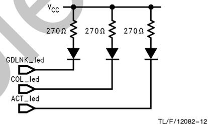
FIGURE 17. Typical DP83907 LED Connection
