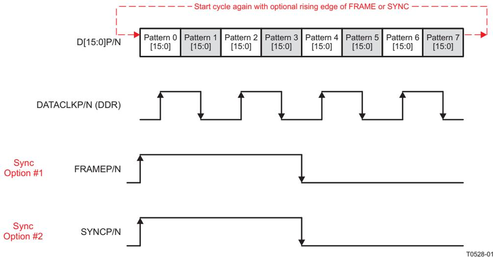
Figure 75. IO Pattern Checker Data Transmission Format
