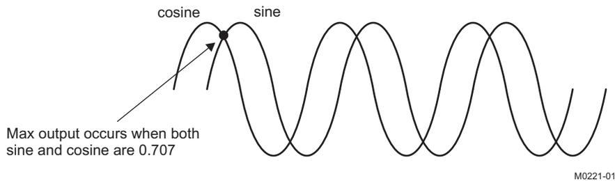
**Figure 72. Maximum Output of the Complex Signal Multiplier**
