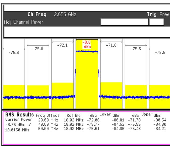
DAC Output IF = 122.88 MHz, LO = 2532.12 MHz, DAC Clock = DAC3482 On-Chip PLL
