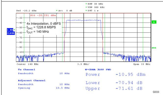
Figure 33. 10 MHz Single Carrier LTE Test Model 3.1
