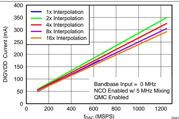
Figure 41. DIGVDD Current vs  $f_{DAC}$  Over Interpolation
