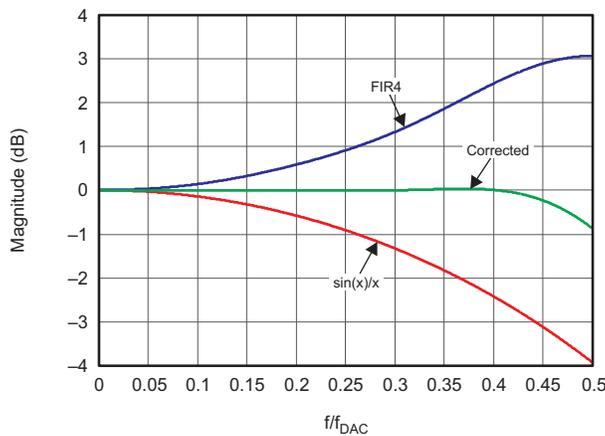
**Figure 68. Magnitude Spectrum for Inverse Sinc Filter**
