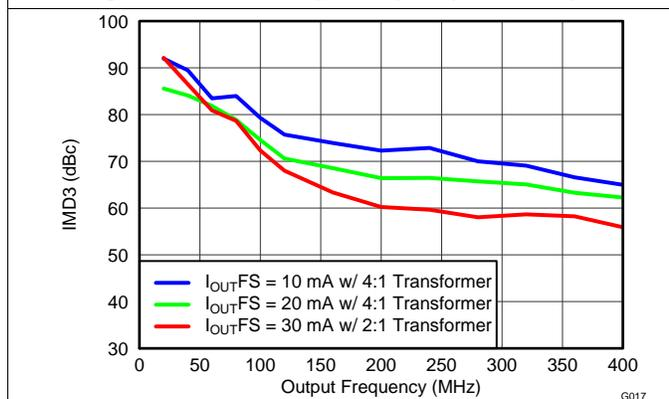
Figure 17. IMD3 vs Output Frequency Over  $I_{OUTFS}$
