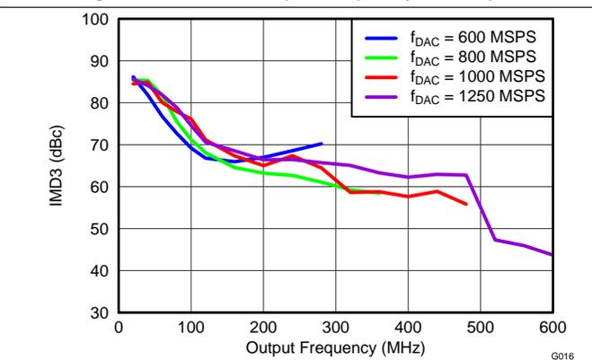
Figure 16. IMD3 vs Output Frequency Over  $f_{DAC}$
