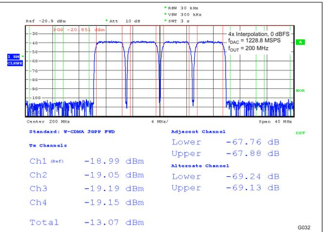
Figure 32. Four Carrier W-CDMA Test Model 1
