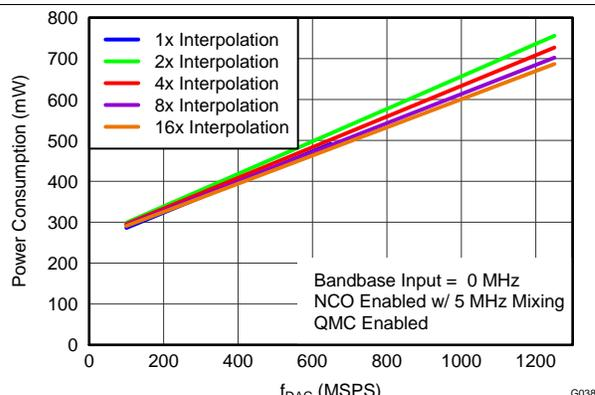
Figure 38. Power Consumption vs  $f_{DAC}$  Over Interpolation
