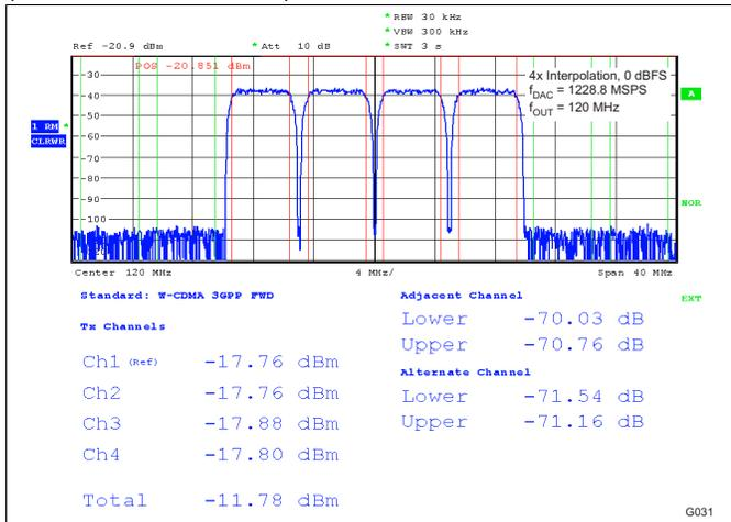
Figure 31. Four Carrier W-CDMA Test Model 1
