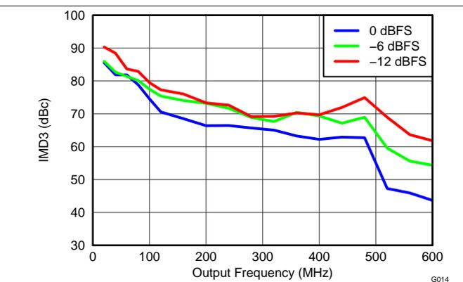
Figure 14. IMD3 vs Output Frequency Over Input Scale
