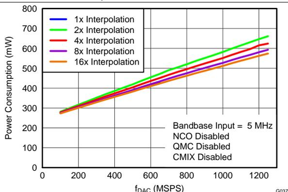
Figure 37. Power Consumption vs  $f_{DAC}$  Over Interpolation
