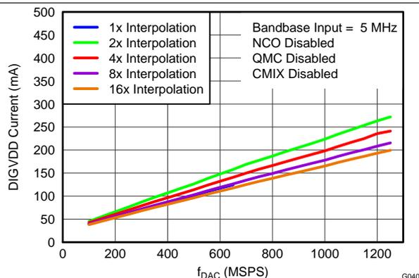
Figure 40. DIGVDD Current vs  $f_{DAC}$  Over Interpolation
