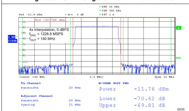
Figure 35. 20 MHz Single Carrier LTE Test Model 3.1
