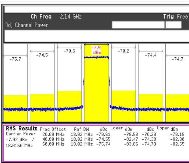
DAC Output IF = 122.88 MHz, LO = 2017.12 MHz, DAC Clock = DAC3482 On-Chip PLL
