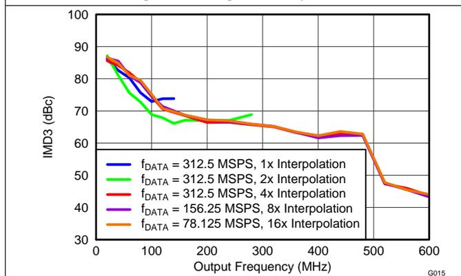
Figure 15. IMD3 vs Output Frequency Over Interpolation
