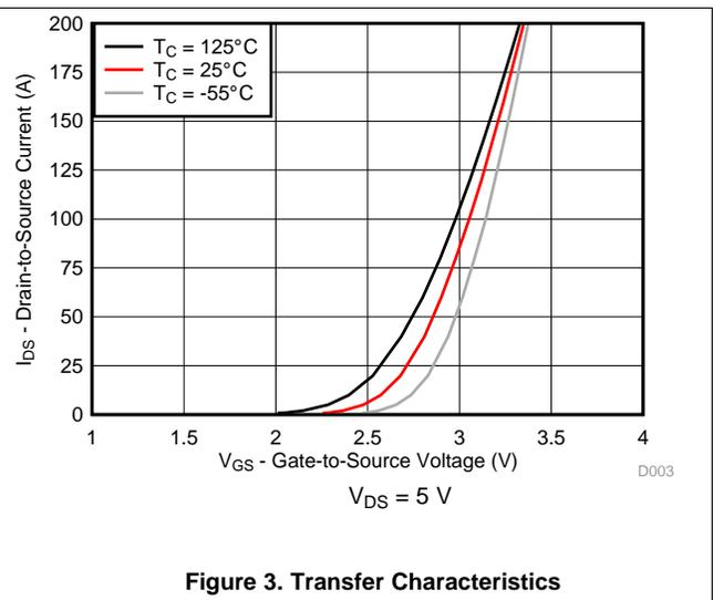
Figure 3. Transfer Characteristics
