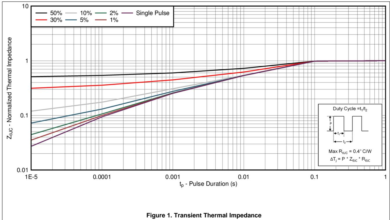
Figure 1. Transient Thermal Impedance
