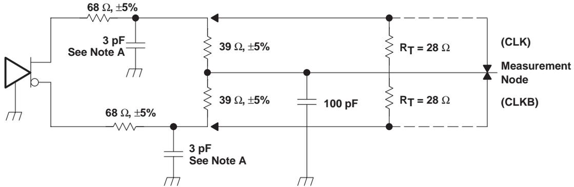
NOTE A: These capacitors represent parasitic capacitance. No discrete capacitors are used on the test board during device characterization.
