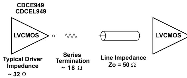
**Figure 2. Test Load for 50 Ω Board Environment**
