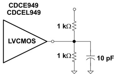
**Figure 1. Test Load**
