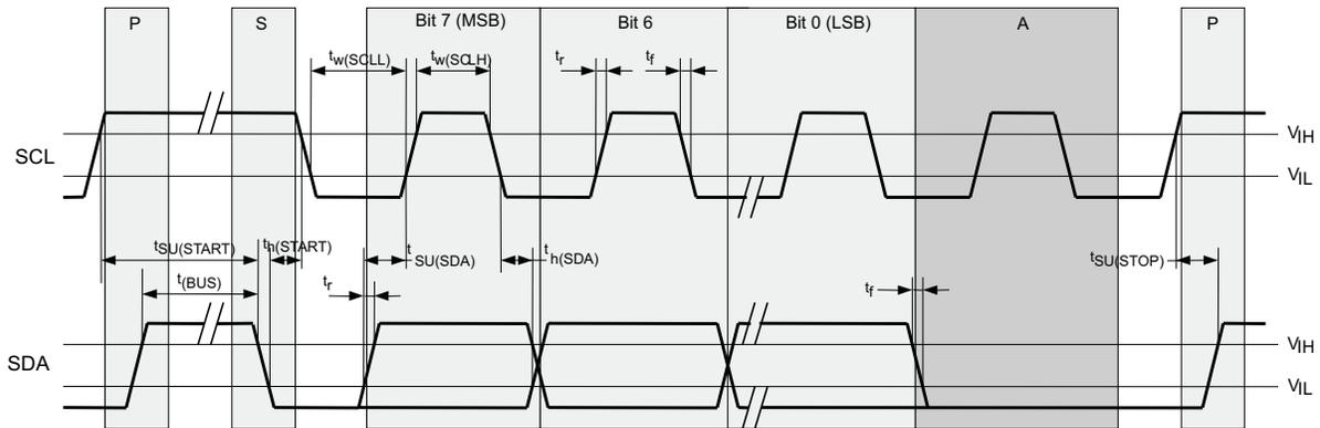
Figure 11. Timing Diagram for the SDA/SCL Serial Control Interface
