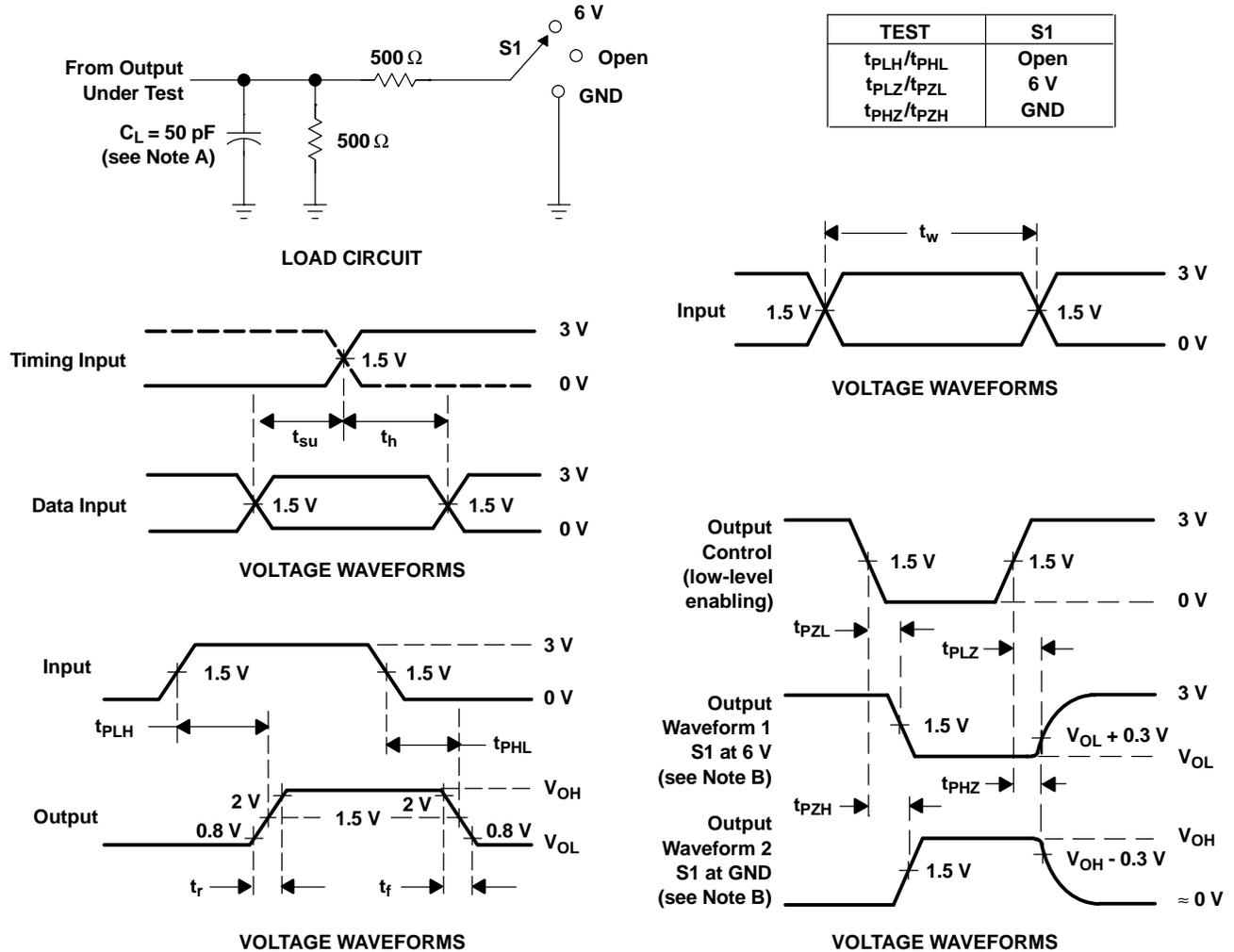
A.  $C_L$  includes probe and jig capacitance.
