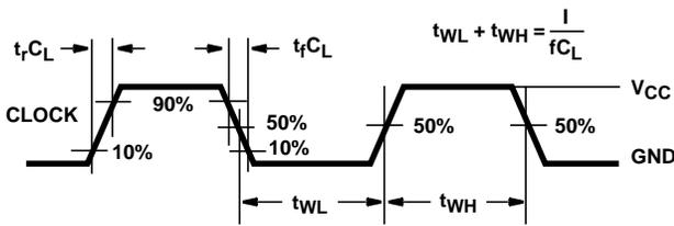
NOTE: Outputs should be switching from 10% V<sub>CC</sub> to 90% V<sub>CC</sub> in accordance with device truth table. For f<sub>MAX</sub>, input duty cycle = 50%.
