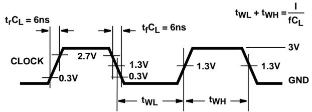
NOTE: Outputs should be switching from 10% V<sub>CC</sub> to 90% V<sub>CC</sub> in accordance with device truth table. For f<sub>MAX</sub>, input duty cycle = 50%.
