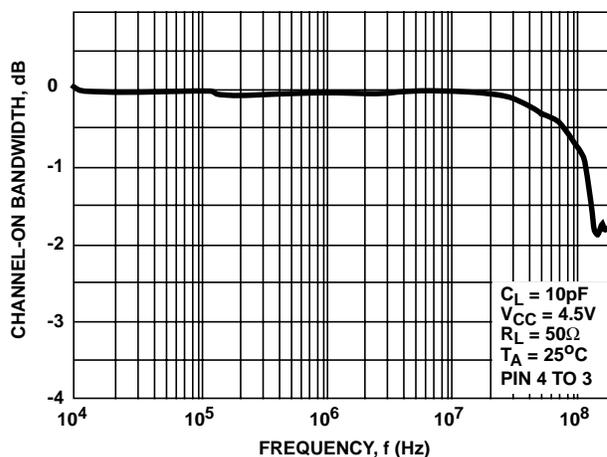
FIGURE 2. SWITCH FREQUENCY RESPONSE,  $V_{CC} = 4.5\text{V}$
