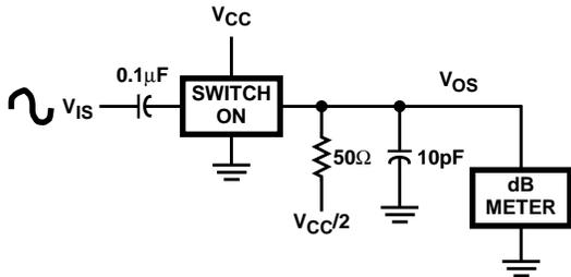
FIGURE 6. TOTAL HARMONIC DISTORTION TEST CIRCUIT
