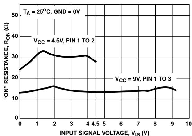
FIGURE 1. TYPICAL "ON" RESISTANCE vs INPUT SIGNAL VOLTAGE
