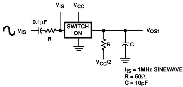
FIGURE 4. CROSTALK BETWEEN TWO SWITCHES TEST CIRCUIT
