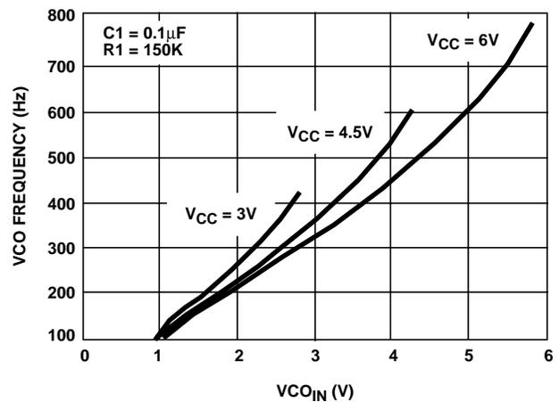
FIGURE 18. HC4046A TYPICAL VCO FREQUENCY vs VCO<sub>IN</sub> (R1 = 150kΩ, C1 = 0.1μF)
