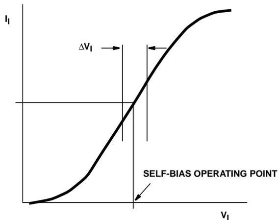
FIGURE 10. TYPICAL INPUT RESISTANCE CURVE AT  $SIG_{IN}$ ,  $COMP_{IN}$
