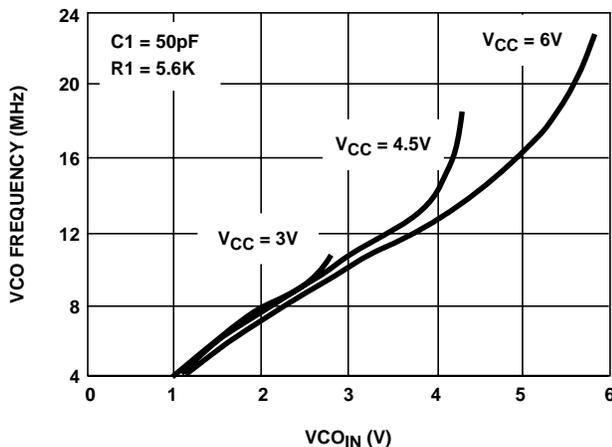
FIGURE 21. HC4046A TYPICAL VCO FREQUENCY vs VCO<sub>IN</sub> (R1 = 5.6kΩ, C1 = 50pF)
