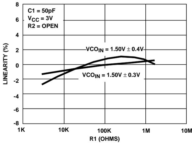
FIGURE 35. HC4046A VCO LINEARITY vs R1 ( $V_{CC} = 3V$ )
