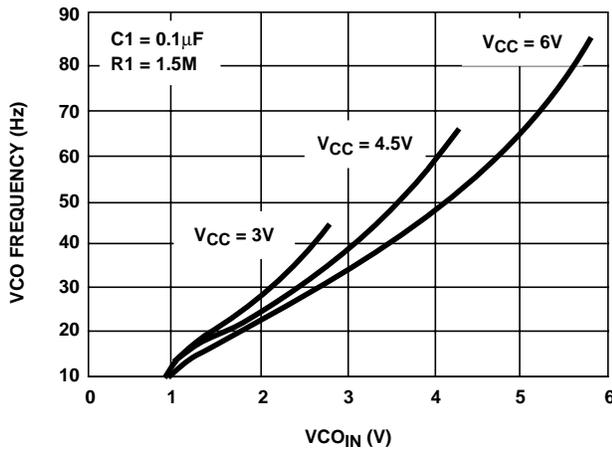
FIGURE 17. HC4046A TYPICAL VCO FREQUENCY vs VCO<sub>IN</sub> (R1 = 1.5MΩ, C1 = 0.1μF)
