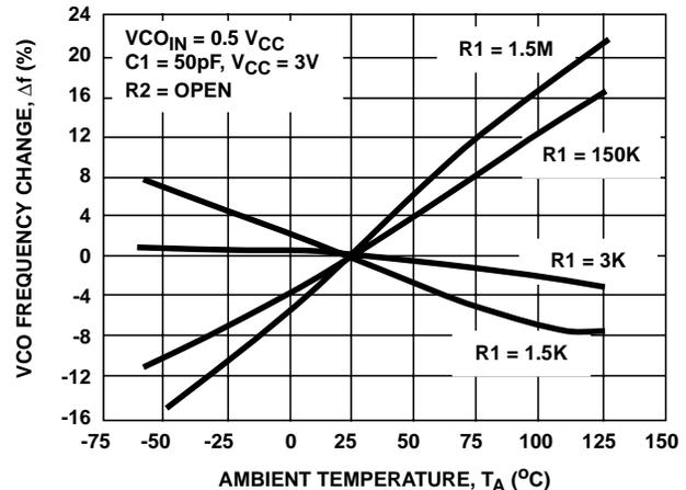
FIGURE 22. HC4046A TYPICAL CHANGE IN VCO FREQUENCY vs AMBIENT TEMPERATURE AS A FUNCTION OF R1 (V<sub>CC</sub> = 3V)
