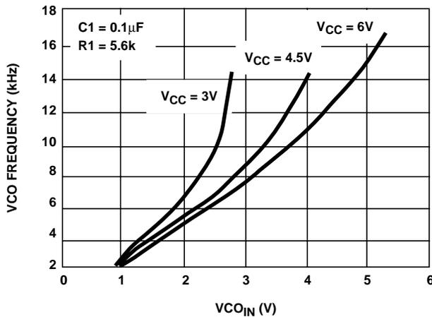
FIGURE 19. HC4046A TYPICAL VCO FREQUENCY vs VCO<sub>IN</sub> (R1 = 5.6kΩ, C1 = 0.1μF)
