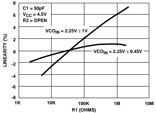
FIGURE 34. HC4046A VCO LINEARITY vs R1 ( $V_{CC} = 4.5V$ )
