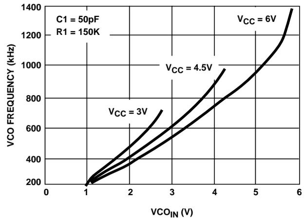
FIGURE 20. HC4046A TYPICAL VCO FREQUENCY vs VCO<sub>IN</sub> (R1 = 150kΩ, C1 = 50pF)
