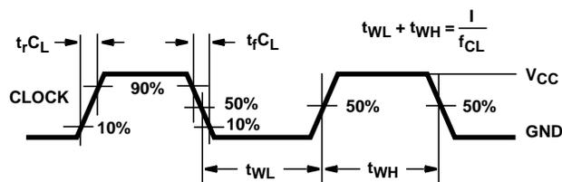
NOTE: Outputs should be switching from 10%  $V_{CC}$  to 90%  $V_{CC}$  in accordance with device truth table. For  $f_{MAX}$ , input duty cycle = 50%.
