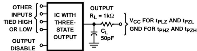
NOTE: Open drain waveforms  $t_{PLZ}$  and  $t_{PZL}$  are the same as those for three-state shown on the left. The test circuit is Output  $R_L = 1k\Omega$   $V_{CC}$ ,  $C_L = 50pF$ .
