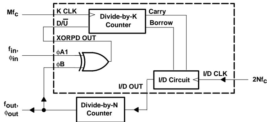
**Figure 2. DPLL Using Exclusive-OR Phase Detection**
