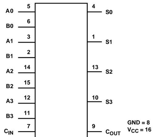
CAUTION: These devices are sensitive to electrostatic discharge. Users should follow proper IC Handling Procedures.
