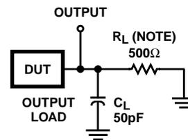
NOTE: For AC Series Only: When  $V_{CC} = 1.5\text{V}$ ,  $R_L = 1\text{k}\Omega$ .
