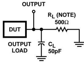
NOTE: For AC Series Only: When  $V_{CC} = 1.5V$ ,  $R_L = 1kΩ$ .
